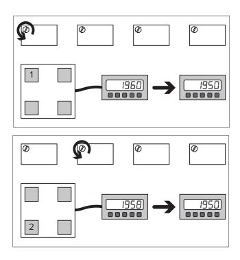
Calibrate the scale with a sample weight and verify again that all the corners display the same weight.
