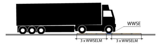
NOTES: The best weighing condition is obtained by creating a levelling area of a length equal to double that of the longest vehicle to be weighed.
