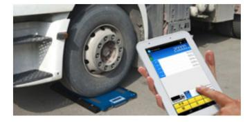
In the example, an application with wireless platform, WWSDUAL option, analogue platform, Bluetooth BLTH and DINI SMART AXLE weighing App.
